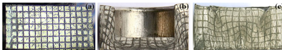
Fig. 5 a The deformation mesh at initial state; and the deformed mesh at the end of b step one, and c step two of ABE process
